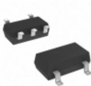
74LX1G04CTR STMicroelectronics IC INVERTER SGL CMOS LV SOT23-5
