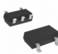
74LX1G07CTR STMicroelectronics IC BUFF DVR N-INV O/DRAIN SC70-5
