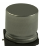
EEV-FK1H471M Panasonic Electronic Components CAP ALUM 470UF 20% 50V SMD
