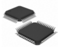
MB90F387SPMT-GS-N2E1 Cypress Semiconductor IC MCU 16BIT 64KB FLASH 48LQFP
