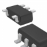
XC6124E742MR-G Torex Semiconductor Ltd IC WATCHDOG TIMER SOT-25
