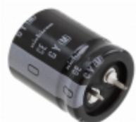
LGY2W680MELA Nichicon CAP ALUM 68UF 20% 450V SNAP
