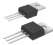
IXYP15N65C3 IXYS IGBT 650V 38A 200W TO220
