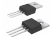
IXYP15N65C3D1 IXYS IGBT 650V 38A 200W TO220
