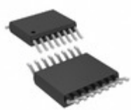
LTC2368HMS-18#TRPBF Linear Technology IC ADC 18BIT 1MSPS SPI 16MSOP
