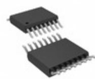
LTC2368HMS-18#PBF ADI (Analog Devices, Inc.) IC ADC 18BIT 1MSPS SPI 16MSOP
