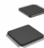
MB90F428GCPMC-G Cypress Semiconductor Corp IC MCU 16BIT 128KB FLASH 100LQFP
