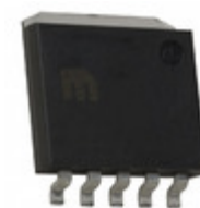
MIC37301-2.5WR Microchip Technology IC REG LDO 2.5V 3A SPAK-5
