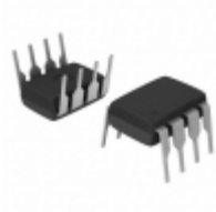
AT25080A-10PU-2.7 Microchip Technology IC EEPROM 8KBIT 20MHZ 8DIP
