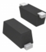
CPDQ3V3U-HF Comchip Technology TVS DIODE 3.3VWM 10.4VC SOD923F
