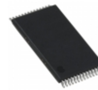
AS6C6264-55STCNR Alliance Memory, Inc. IC SRAM 64KBIT 55NS 28TSOP
