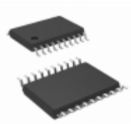
MC74VHCT541ADTG ON Semiconductor IC BUFF/DVR 8BIT N-INV 20TSSOP
