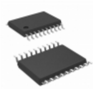
MC74VHCT541ADT ON Semiconductor IC BUFF/DVR 8BIT N-INV 20TSSOP
