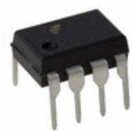
FAN7711SN Fairchild/ON Semiconductor IC BALLAST CTRL ELECTR 8-DIP
