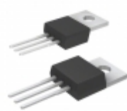
IXTP230N075T2 IXYS MOSFET N-CH 75V 230A TO-220
