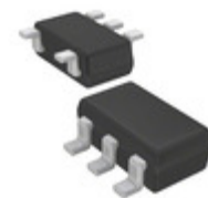
ADM6320CZ29ARJ-RL7 Analog Devices Inc. IC SUPERVISOR WATCHDOG SOT23-5
