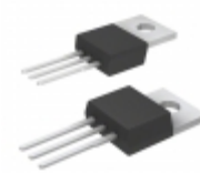
IXCP20M35 IXYS IC CURRENT REGULATOR TO220AB
