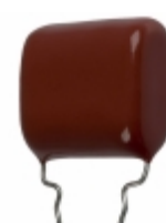
ECQ-P1H274FZW Panasonic Electronic Components CAP FILM 0.27UF 1% 50VDC RADIAL
