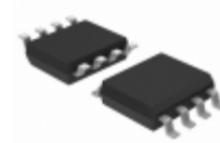
SST25VF040B-80-4I-S2AE-T Microchip Technology IC FLASH 4MBIT 80MHZ 8SOIC
