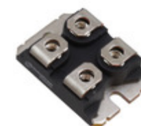
GSXF060A120S1-D3 Global Power Technologies Group DIODE FAST REC 1200V 60A SOT227
