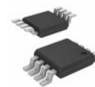
MIC3775-3.0YMM Microchip Technology IC REG LDO 3V 0.75A 8MSOP
