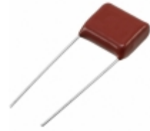
ECQ-E6224RJ Panasonic Electronic Components CAP FILM 0.22UF 5% 630VDC RADIAL
