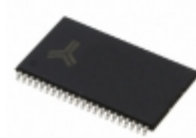
AS7C34098A-12TIN Alliance Memory, Inc. IC SRAM 4MBIT 12NS 44TSOP
