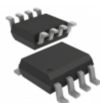
OP293FS-REEL Analog Devices Inc. IC OPAMP GP 35KHZ RRO 8SOIC
