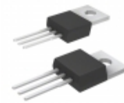
IXTP1R4N120P IXYS MOSFET N-CH 1200V 1.4A TO-220
