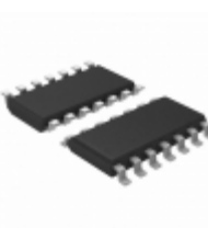
AD8044ARZ-14-REEL7 Analog Devices Inc. IC OPAMP VFB 160MHZ RRO 14SOIC
