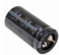
LGX2G391MELA50 Nichicon CAP ALUM 390UF 20% 400V SNAP
