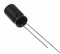
EEU-FC1A151B Panasonic Electronic Components CAP ALUM 150UF 20% 10V RADIAL
