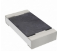
RC1206FR-07140RL Yageo RES SMD 140 OHM 1% 1/4W 1206
