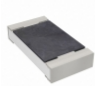
RC1206FR-0714K3L Yageo RES SMD 14.3K OHM 1% 1/4W 1206
