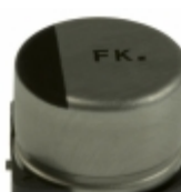
EEE-FK1A471GP Panasonic Electronic Components CAP ALUM 470UF 20% 10V SMD
