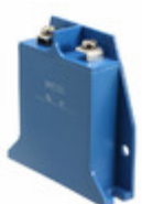
B72260B0251K001 EPCOS VARISTOR 390V 70KA CHASSIS
