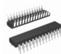
PIC16LC773-I/SP Microchip Technology IC MCU 8BIT 7KB OTP 28SDIP
