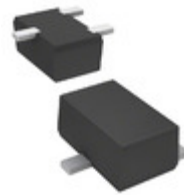
DSC5002R0L Panasonic Electronic Components TRANS NPN 50V 0.5A SMINI3
