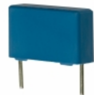
B32652A0103J289 EPCOS CAP FILM 10000PF 5% 1KVDC RADIAL
