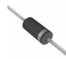
BZW06-15 A0G TSC (Taiwan Semiconductor) TVS DIODE 15.3V 32.5V DO204AC
