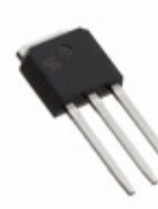
TSM80N1R2CH C5G TSC (Taiwan Semiconductor) MOSFET N-CH 800V 5.5A TO251
