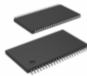
71V424S10PHG IDT, Integrated Device Technology Inc IC SRAM 4MBIT 10NS 44TSOP
