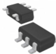
XC6122C242MG-G Torex Semiconductor Ltd IC WATCHDOG TIMER SOT-25
