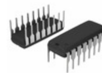
DG542DJ-E3 Electro-Films (EFI) / Vishay IC SWITCH QUAD SPST 16DIP
