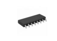
HEF4046BT,653 Nexperia IC PHASE LOCK LOOP W/VCO 16SOIC
