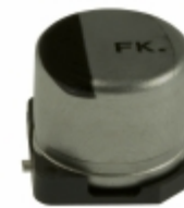
EEV-FK1V101XP Panasonic Electronic Components CAP ALUM 100UF 20% 35V SMD
