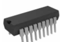
PIC16C622A-20/P Microchip Technology IC MCU 8BIT 3.5KB OTP 18DIP
