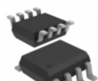
AMP03GSZ Analog Devices Inc. IC OPAMP DIFFERENTIAL 3MHZ 8SOIC
