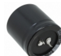
LGN2E102MELC35 Nichicon CAP ALUM 1000UF 20% 250V SNAP
