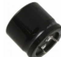
LGN2E102MELB40 Nichicon CAP ALUM 1000UF 20% 250V SNAP
