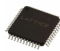
ISPLSI 2064VE-135LT44 Lattice Semiconductor Corporation IC CPLD 64MC 7.5NS 44TQFP
