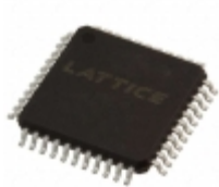
ISPLSI 2064VE-135LTN44 Lattice Semiconductor Corporation IC CPLD 64MC 7.5NS 44TQFP
