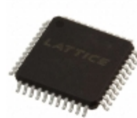
ISPLSI 2064VE-135LTN44I Lattice Semiconductor Corporation IC CPLD 64MC 7.5NS 44TQFP
