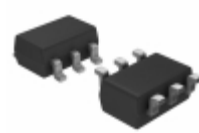
93LC46AT-E/OT Microchip Technology IC EEPROM 1KBIT 2MHZ SOT23-6
