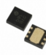
XC6122E544ER-G Torex Semiconductor Ltd IC WATCHDOG TIMER 6-USP
