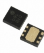
XC6122E545ER-G Torex Semiconductor Ltd IC WATCHDOG TIMER 6-USP
