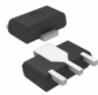
AN77L045M Panasonic IC REG LDO 4.5V 0.1A 3HSIP
