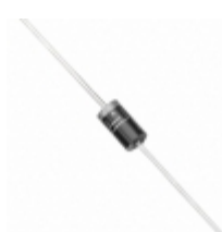
1.5KE36A Littelfuse Inc. TVS DIODE 30.8VWM 49.9VC AXIAL
