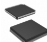
AT40K05-2CQI Microchip Technology IC FPGA 5K GATES 160QFP
